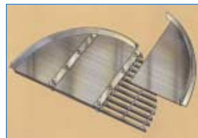
In retrofitting fixed bed systems, damaged wire mesh is removed, leaving still-serviceable support grating in place. Johnson screens are then installed over the grating, creating a very strong, efficient and long-lasting system.
